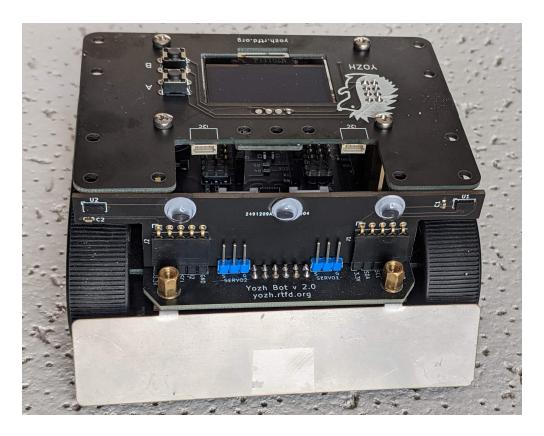
Yozh is a small (under 10cm\*10cm) robot, based on Pololu's Zumo chassis. It was created by shurik179 for a robotics class at SigmaCamp. Below are the key features of this robot.
