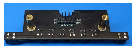
3. Plug the reflectance array into the female header at the bottom of the robot main board. Pull it slightly out so that there is a small gap (about 1mm) between the top of the standoff and the bottom of the main board.
