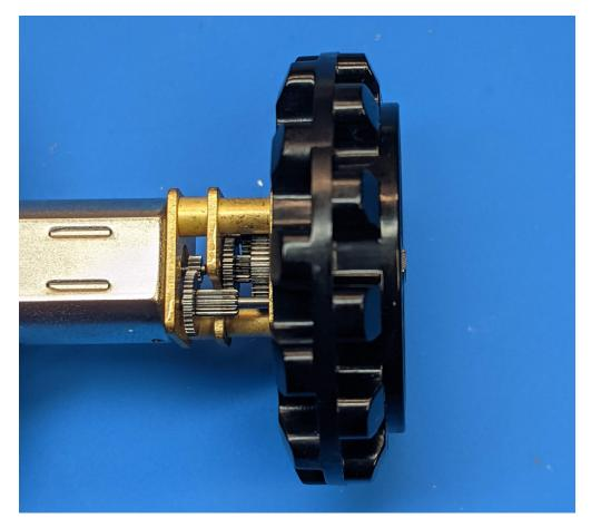
Place the motors on the table, using sprockets as supports, and solder the motor leads to each motor. (You probably want to use a third hand or similar device to support the wires while soldering.)
